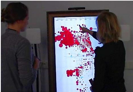
**Figure 1.** Two people interacting with our system prototype. A 65" display is used in combination with two RFID antennas (left and right side) and one *Kinect*<sup>TM</sup> camera (on top)
